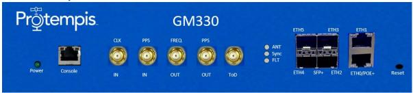
The RJ45 console serial port provides an interface with up to 230k bits/sec to the Time serve.
