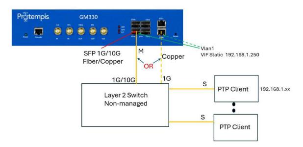
If you plan on connecting an external Layer 2 switch, make sure you are not creating a loop. Currently, the GM330 does not support spanning tree. This feature will be introduced in future firmware.
