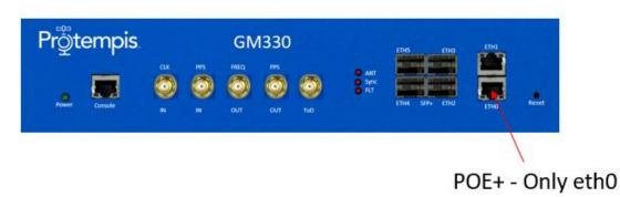
Note - When switching the power from DC to POE the unit will reset (POE is not "hot standby" power). Switching from POE to DC should be seamless.
