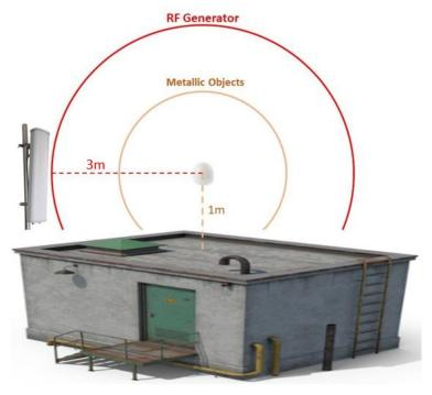
NOTE - GNSS antenna should be at least one meter away from any metallic objects to avoid multipath reflections.
