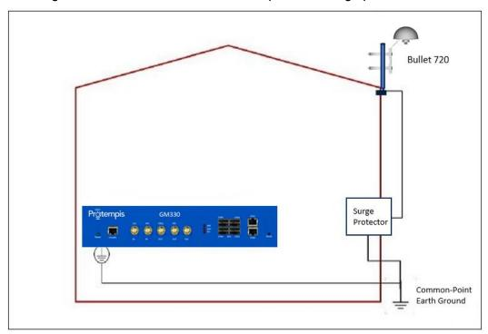
It is recommended to use a minimum of 6 AWG (13.3 mm) wire or larger.
