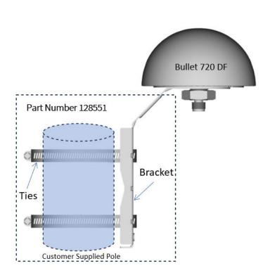
The thread specification of the Bullet antenna is a 3/4" NPT thread, dimensions according to ANSI/ASME B1.20.1. It is also called a 1"-14 marine thread because it has 14 threads per inch
