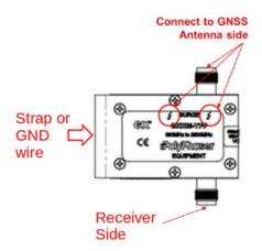
The image below shows the direction of the coaxial cable connection between the GNSS antenna and the Time server.
