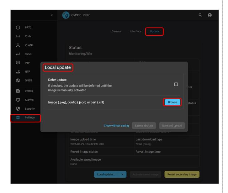
Once \*.crt is selected click on "Save and Upload". Confirm the file was uploaded successfully by Looking at the "image verify status" field as shown below.
